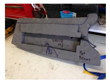
If you haven't cut your bulkhead yet, and don't want to modify it, you can simply get some foam and attach a 2-inch chunk on top and bottom or a 4-inch chunk up top. Super simple.
